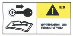
When the machine is maintained, turn off the engine and pulled out the key This sing is posted at the engine switch
