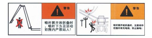
When the spray rod is unfolded and folded, it is strictly prohibited to stand below. This sign is posted on the spray rod.
