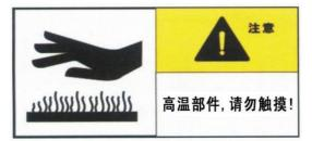
High temperature, do not touch. This sign is posted at the engine exhaust pipe
