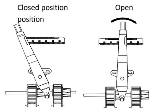
You can set the amount of seed you will plant in accordance with the following table by means of the Seed and Fertilizer Setting Lever.
