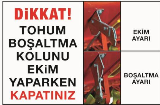
**It is ensured that seeds are discharged by working simultaneously through the lever controlling the couplings of the seed and fertilizer maws.**
