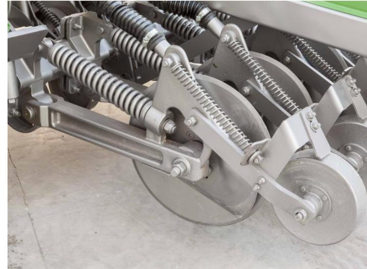
The pin on the shaft is used for increasing this pressure.
