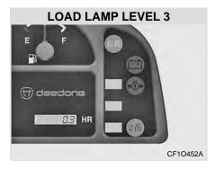
Load lamp + 3 lamps illuminated: deceleration desired
