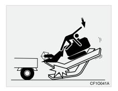
Use ramps that are strong, wide and long (4 times long as the height of the cargo bed of the vehicle) enough and have anti-slippery hooks.
