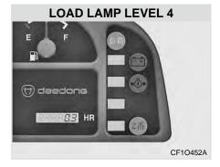
Load lamp + 4 lamps illuminated: immediate deceleration required
