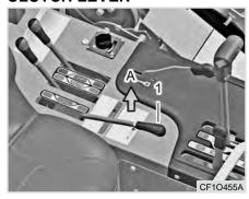
(1) Reaping Unit Reversing Clutch Lever (A) Up
