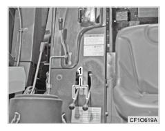
(1) Reaping / Threshing Clutch Lever
