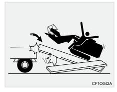
Ensure the ramps are straightly lined up with the cargo bed of the transporting vehicle.
