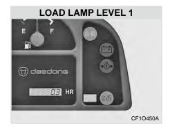
Load lamp + 1 lamp illuminated: acceleration possible
