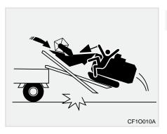
Do not operate any shift or the steering lever on the ramps.
