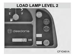
Load lamp + 2 lamps illuminated: current speed appropriate
