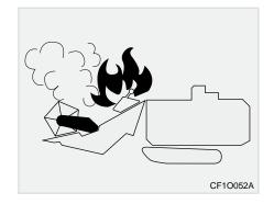
Do not run the engine with the body, cutter, binder, dust-proof cover and grain tank open.
