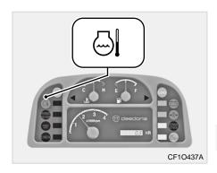
When the engine coolant is excessively hot, this warning lamp blinks and the horn sounds at an interval. To check the coolant, wait until the engine is cooled down. Then, open the radiator pressure cap slowly.
