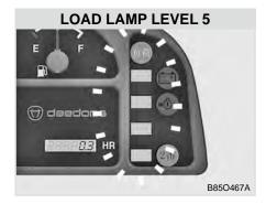
Load lamp + 4 lamps blinking: immediate deceleration required
