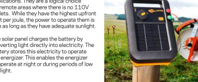
Multi Powered Energizers combined with various adaptors will allow you to power your Energizer using any one of the methods listed above: 110V Outlet, Battery or Solar. This is a great choice if you move your fence to locations where 110v power will exist and other locations where it is not available.
