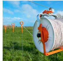
Use an insulated handle on the far end of your portable electric fence so the fence is only powered from one side (at the geared reel). This ensures that the portable fence loses power once you disconnect the alligator clamps and geared reel so you can roll up the wire without getting shocked.
