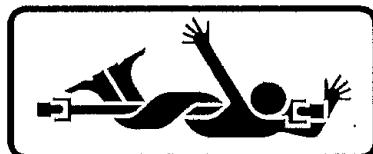
**DANGER:** never get near to the PTO shaft when it is in operation.
