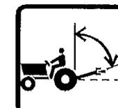
Avoid sharp angulation of drive line as this can damage the pump or the PTO shaft of the tractor.
