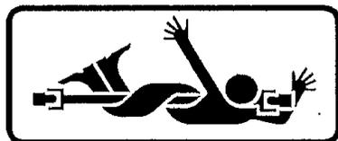
**DANGER:** never get near to the PTO shaft when it is in operation.
