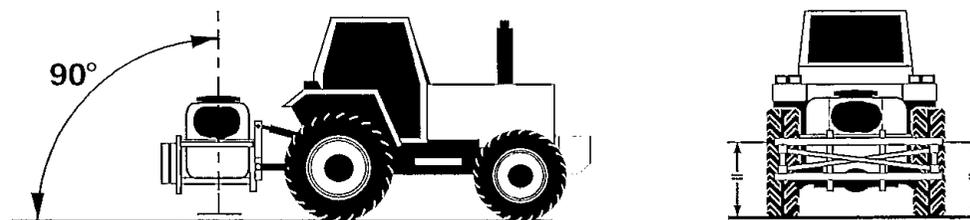
Make sure at least 20% of total weight (tractor+machine working condition) lays on front axle. If not add proper ballast. However, never exceed tyres capacity. Make sure to have lifted and stored any stand leg of which the machine could be provided.
