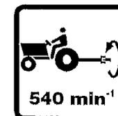
Never run the power take-off at speed exceeding 540 R.P.M. (revolutions per minute).
