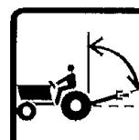
Avoid sharp angulation of drive line as this can damage the pump or the PTO shaft of the tractor.
