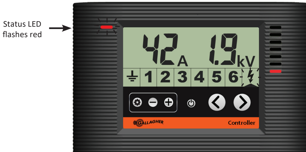
Controller showing the energizer in current alarm
