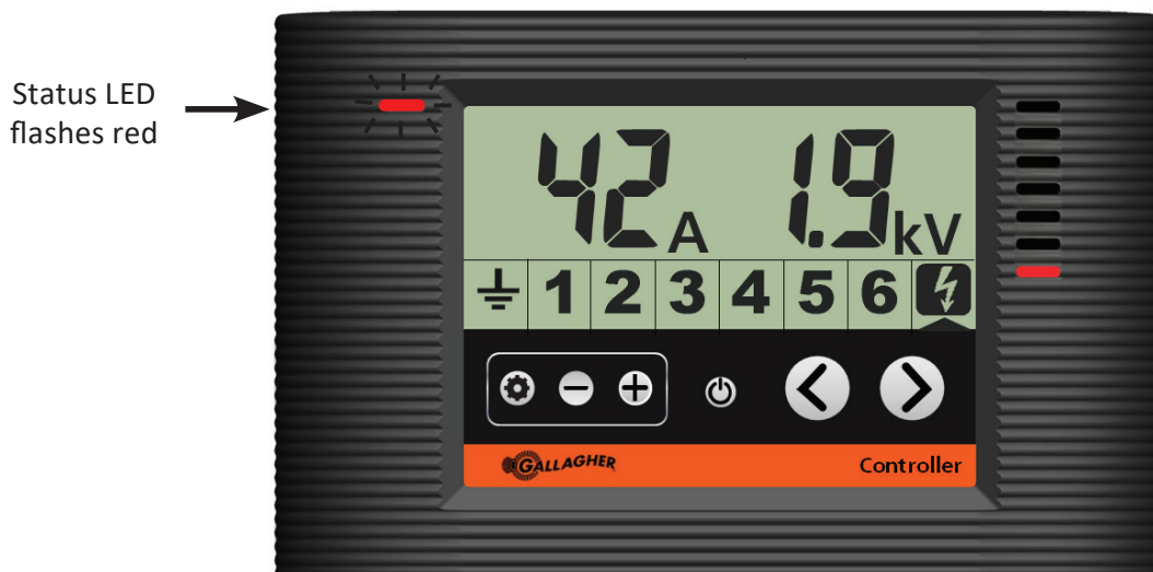
Controller showing the energizer in output alarm
