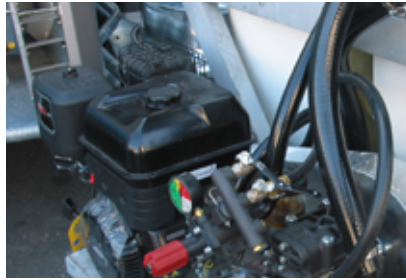
4 stroke engine made Briggs-Straton 14 HP gasoline fuel
