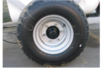
Tubed wheels 11.5/80 - 15.3 mounted on 6x6 hub and adjustable axles equipped of conic bearings of first class
