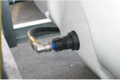
Jet agitation to mix the chemical and to maintain the concentrations of the mixture during the spraying phases
