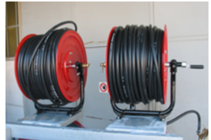
Hose reel with 100 meters hose 10x19 80 Bar
