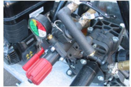
Pressure regulation valve with cock valve to command the jet agitations and gauge
