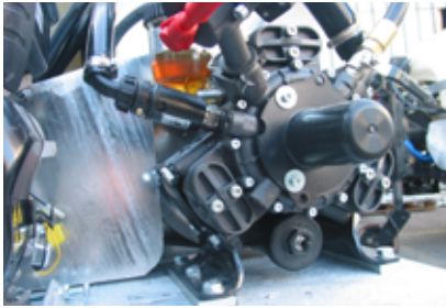
Multi diaphragm pump with safety valve to protect the hydraulic circuit
