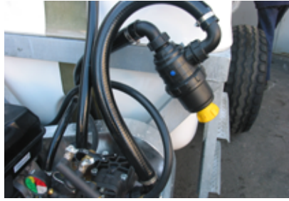
Section filter with shut-off valve, 50 mesh strainer for easy maintenance
