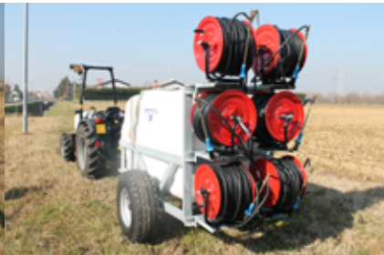
Spraying stations suitable for 6 users and one driver to spray independently the mixture up to 100 meter from the sprayer
