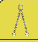
Lifting points are identified by lifting decals. Lifting at other points is unsafe and can damage machinery.
