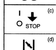
(c). The indication regarding the switch. Flipping the engine switch to the "O" (STOP) direction, the engine stops.
