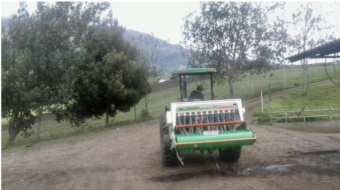
**Fill the hopper (tank) with seed and fertilizer separately.**
