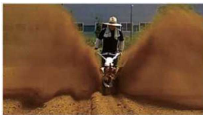
Ditching Rotor(scattering) SDR-200N / 250 / 300 Distance of scattering Max 2.8m(one side)
