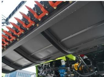
**Header base plate:** Header base plate is made of stainless steel and added with reinforced ribs to the structure to make the header more wear-resistant.
