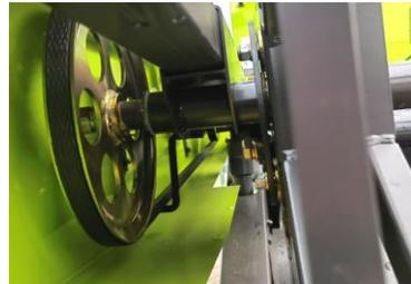
**Header drive:** The reel is driven by belt. Once overload occurs in feeding, the belt slips automatically, which provides an automatic protection.
