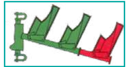
Bivomere trasformabile a trivomere Two furrow plough transf. Into three furrow plough Bisoc transformable en trisoc
