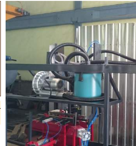
⑦ VACUUM TANK AND MOTOR SHELF
